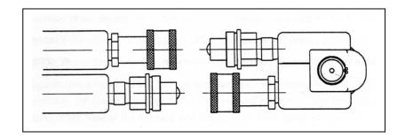
Insure the connectors are fully engaged and screwed snugly together.
